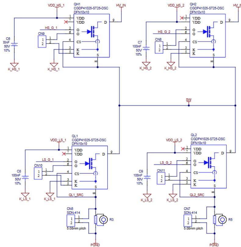
Figure 6 - Half-bridge schematics with paralleled ICeGaN
