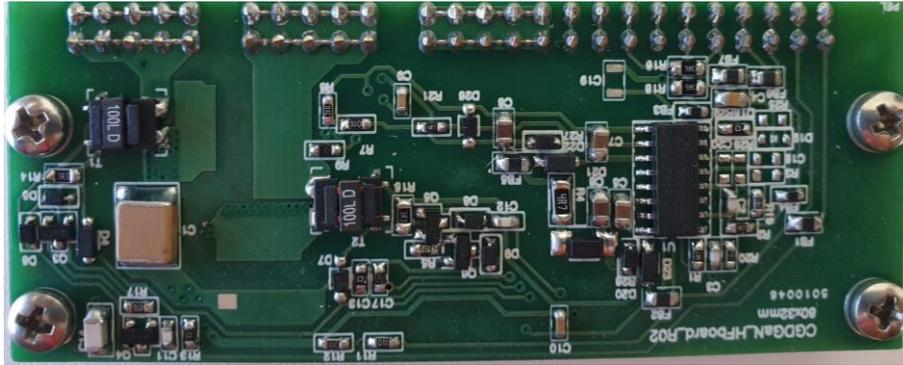
Figure 9 - Top-side cooling example: SMD component side
