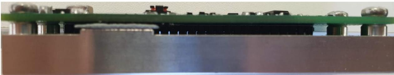
Figure 12 – Top-side cooling heatsink mounted on a PCB
