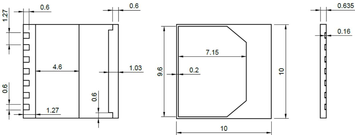
Figure 2 – DHDFN package dimensions in millimetres (mm)
